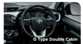
STEERING SWITCH (AUDIO, TELEPHONE, VR, MID) Steering wheel designed for excellent operability, incorporating control switches for audio, telephone, VR, and MID. (V & G Type Double Cabin)
